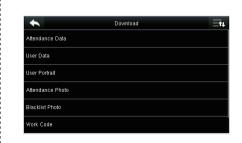
Insert the usb disk correctly, download the attendance data to the disk, then upload that from the disk to your computer. The downloaded data is named "Device Serial Number.dat", you can open and view it.
