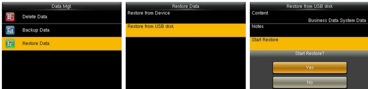
Insert the USB disk. In the initial interface, press [M/OK] > Data Mgt. > Restore Data > Restore from USB Disk > Content > choose content to be restored (Business Data / System Data) > Start Restore > select Yes to start restoring. After restoration completes, click [OK] to automatically restart the device.
