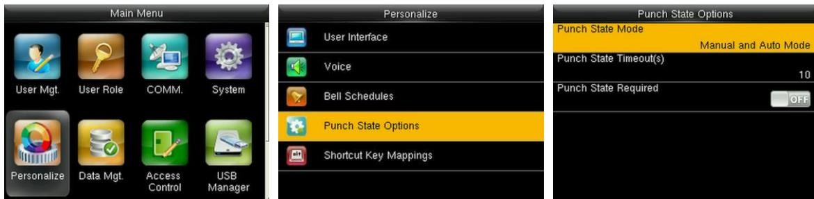
In the initial interface, press [M/OK] > Personalize > Punch State Options to enter the Punch State Options settings interface.
