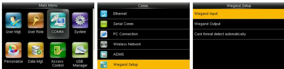
In the initial interface, press [M/OK] > Comm. > Wiegand Setup to enter the Wiegand Setup setting interface.
