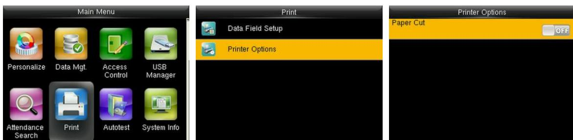
In the initial interface, press [M/OK] > Print > Printer Options > press [M/OK] to turn on / off the Paper Cut function.
