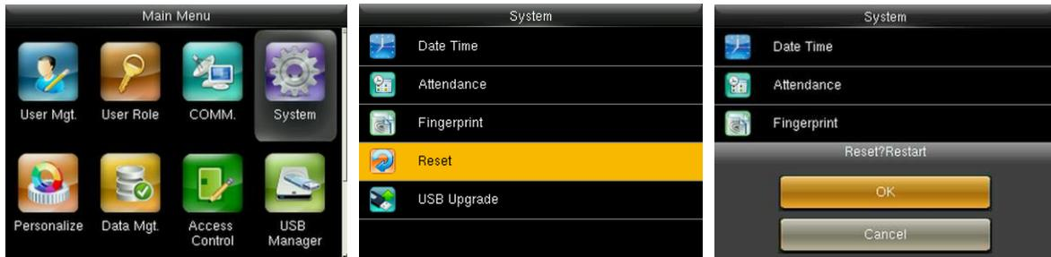
In the initial interface, press [M/OK] > System > Reset > OK to finish the reset setting.
