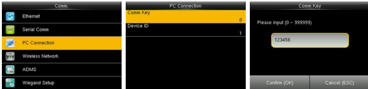
In the initial interface, press [M/OK] > Comm. > PC Connection > Comm Key to enter the Comm Key setting interface.
