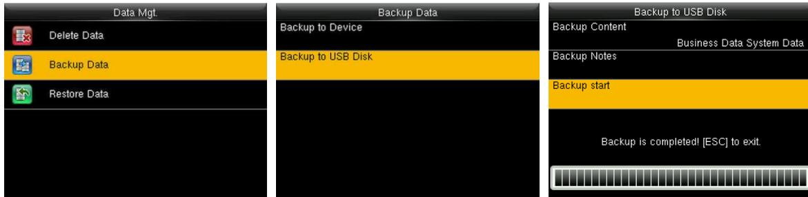
Insert the USB disk. In the initial interface, press [M/OK] > Data Mgt. > Backup Data > Backup to USB Disk > Backup Content > choose content to be backed up (Business Data / System Data) > Backup Start to start backup. Restarting the device is not needed after backup is completed.
