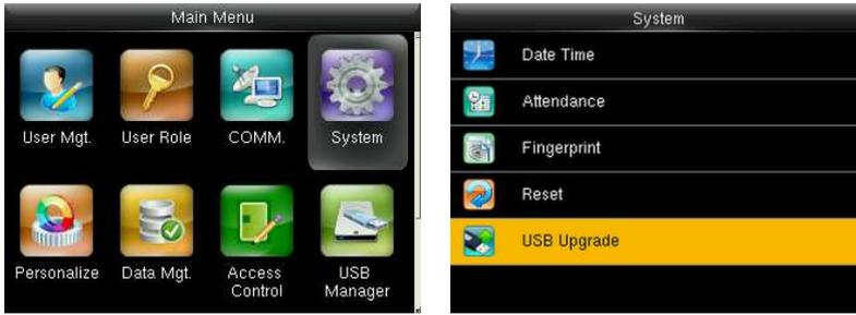
Insert the U disk with upgrade file into the device's USB port, and in the initial interface, press [M/OK] > System > USB Upgrade to complete firmware upgrade operation.
