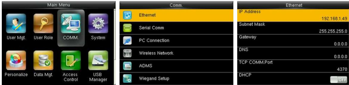
In the initial interface, press [M/OK] > Comm. > Ethernet to enter the Ethernet setting interface.
