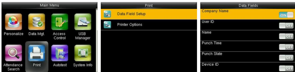
In the initial interface, press [M/OK] > Print > Data Field Setup > press [M/OK] to turn on / off the fields needing to be printed.
