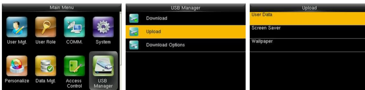
In the initial interface, press [M/OK] > USB Manager > Upload to enter the USB Upload interface.
