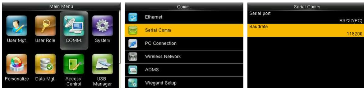
In the initial interface, press [M/OK] > Comm. > Serial Comm > Baudrate to enter the Baudrate setting interface.
