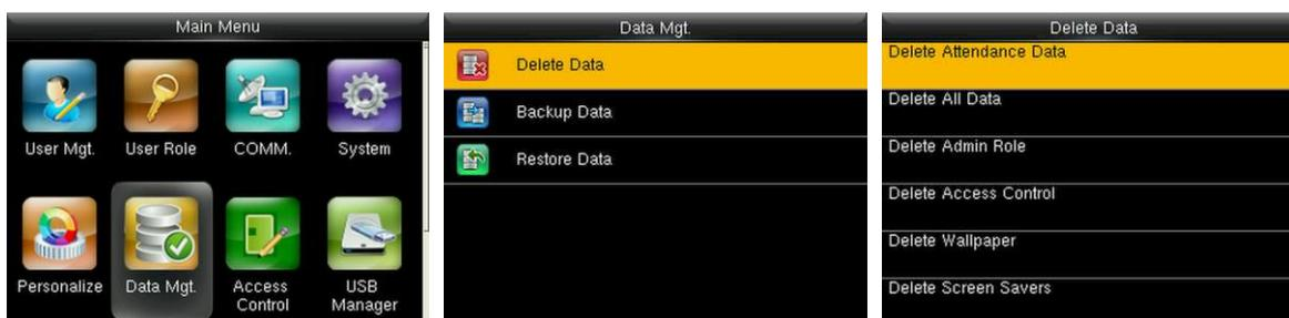
In the initial interface, press [M/OK] > Data Mgt. > Delete Data to enter the Delete Data settings interface.
