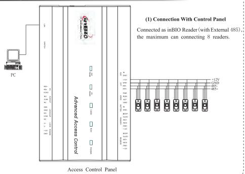
The device can only be used as reader. It cannot dispose the obtained information. Therefore, it needs connecting host machine to obtain fingerprint information and transmit it to host machine for disposal through RS485. The host machine is specified access control terminal which you can consult the commercial representative. Please power off the device before connection. Connection under power-on state may bring great damage to the device.
