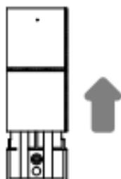
After the battery has been replaced, please put the sensor over the bottom cover and gently slide down to install it.
