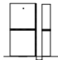
The magnet should be aligned with the middle of sensor and placed within 0.79 inches (2.0 cm) of sensor when the door or window is closed, as shown in the image left.
