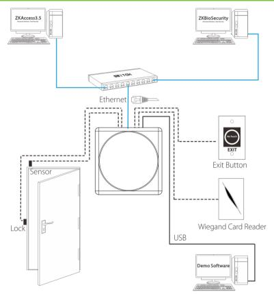
(1)If a registered user verified, the device will export the signal to unlock the door.
