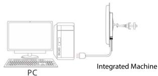
Connect the USB port of the integrated machine to the USB port of the computer. Set the working parameters of the integrated machine using DEMO software.
