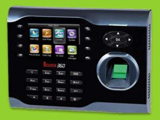
iClock360 is an innovated biometric identification for time attendance application. It can support 8000 fingerprint capacity and 200,000 log capacity, which is suitable for big enterprises.
